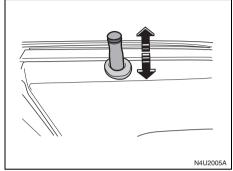
All doors, except the driver's door, can be locked from the outside by pushing down the manual door lock and then closing the door. The driver's door lock cannot be pushed in while the door is open. Upon leaving the vehicle, the driver's door can be locked from the outside only by using the key or the optional remote keyless entry transmitter.
